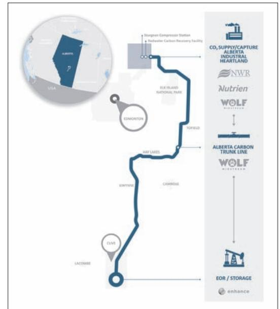
*Alberta Carbon Trunk Line, the world's largest CO<sub>2</sub> pipeline, began operation in 2020 with a capacity of 14.6 million tonnes per year of CO<sub>2</sub>, to connect multiple large-scale CCS projects and sequestration facilities through a transport hub*
