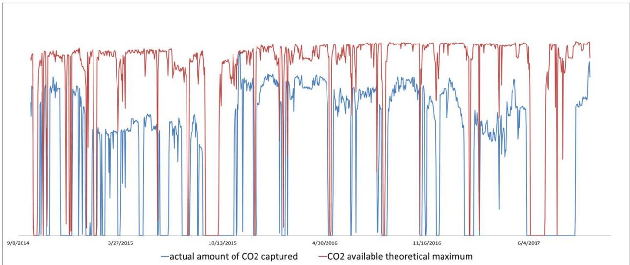
*Figure 1. Comparing actual amount of CO<sub>2</sub> captured and available theoretical maximum CO<sub>2</sub> for capture*
