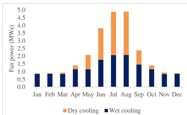
Fig. 5. Fan power consumption
