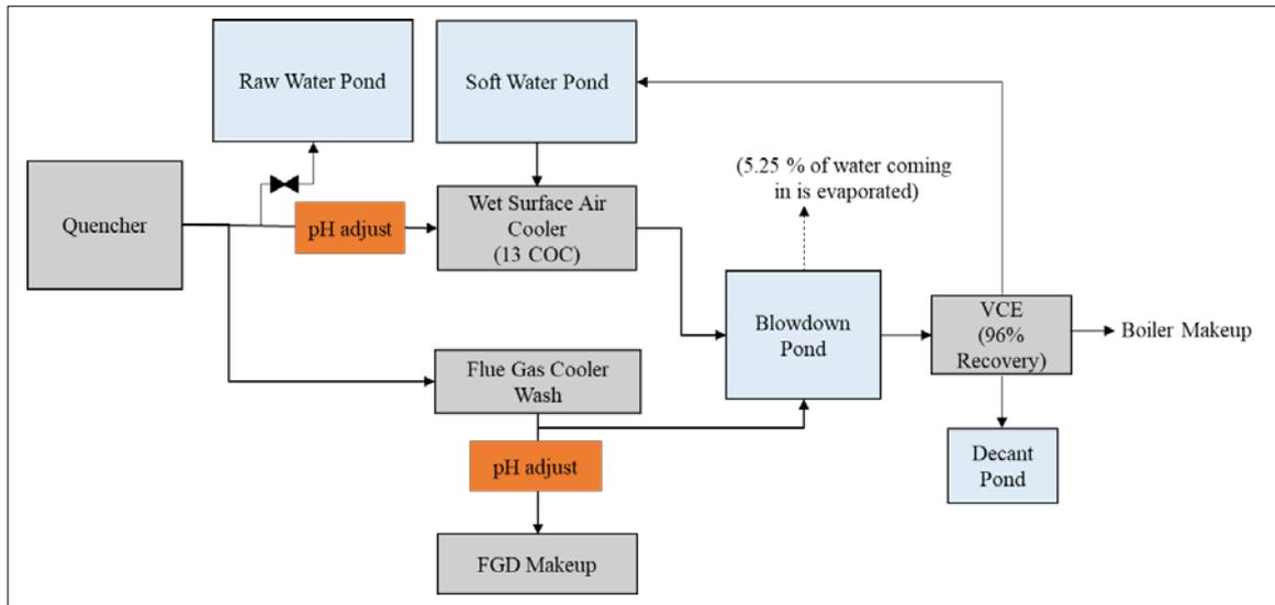
Fig. 1. Simplified diagram of optimized water usage and waste
