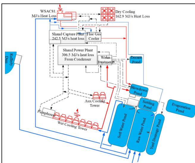
Fig. 2. Shand Power Station integrated CCS water balance
