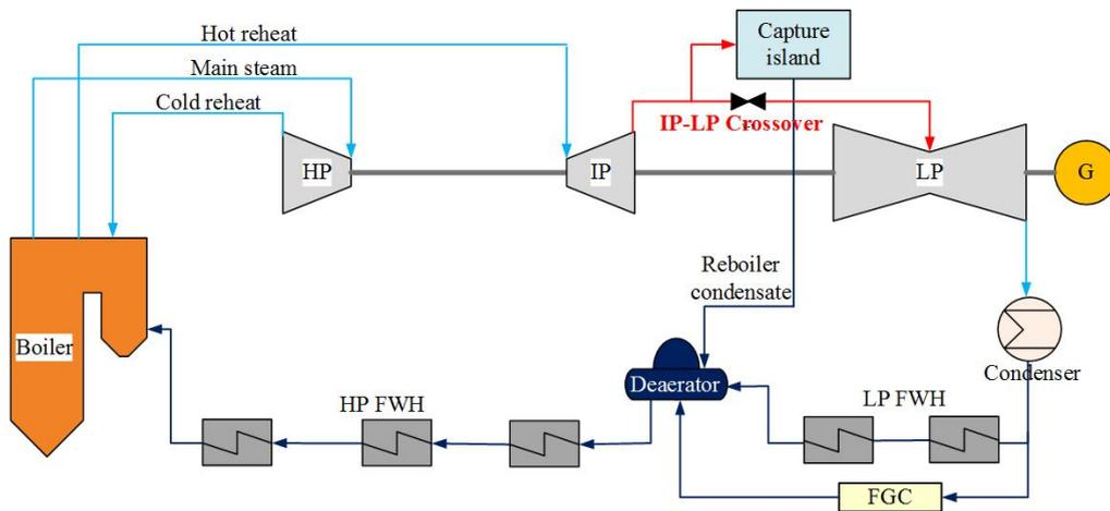
Figure 1. Controlled steam extraction from cross-over
