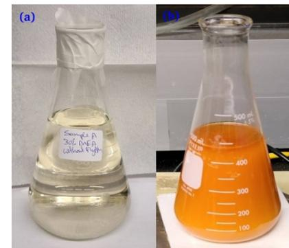
Fig. 3. 30 wt.% MEA sample (323.15 K, after 120 hours of air flow); (a) 30 wt.% MEA without Fly ash, and (b) 30 wt.% MEA with 0.5 wt% of fly ash
