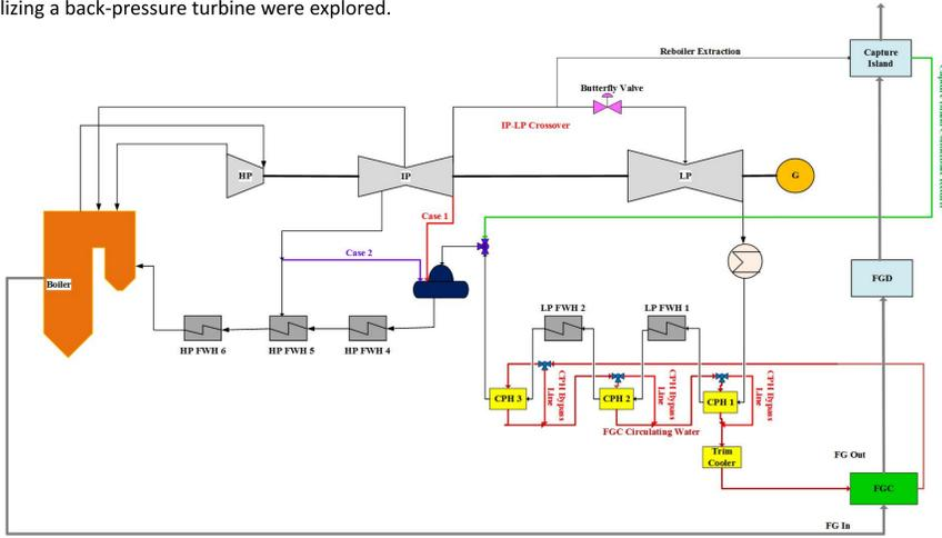
Figure 1. Steam Cycle Configurations for Reboiler and DEA Extractions
