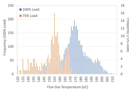
Figure 4. Histogram summarizing flue gas stack temperatures at 100% and 75% Loads
