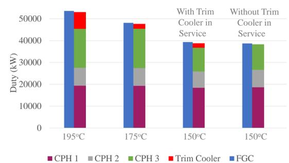
Figure 6. Summary of FGC and CPH loop duties at varying FG temperatures
