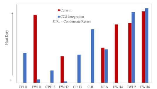
Figure 7. Comparing the associated duty for each component in the feed heating train between the current and CCS integrated cases
