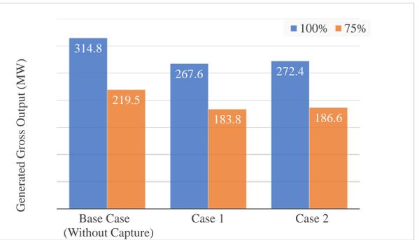
Figure 2. Comparing gross output between the base case, case 1 and case 2
