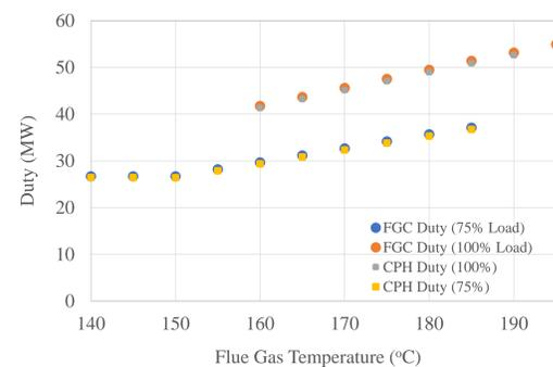
Figure 5. Summary of FGC and CPH duty with varying flue gas temperatures at 100% and 75% loads
