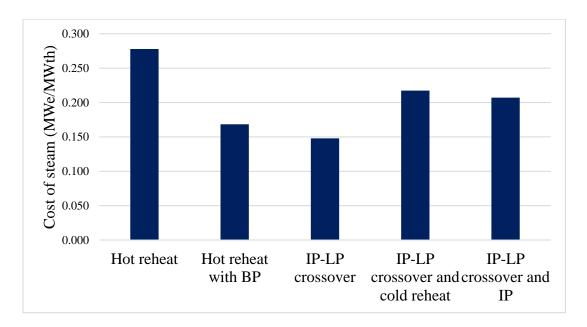
Figure 1. Cost of steam at different extraction
