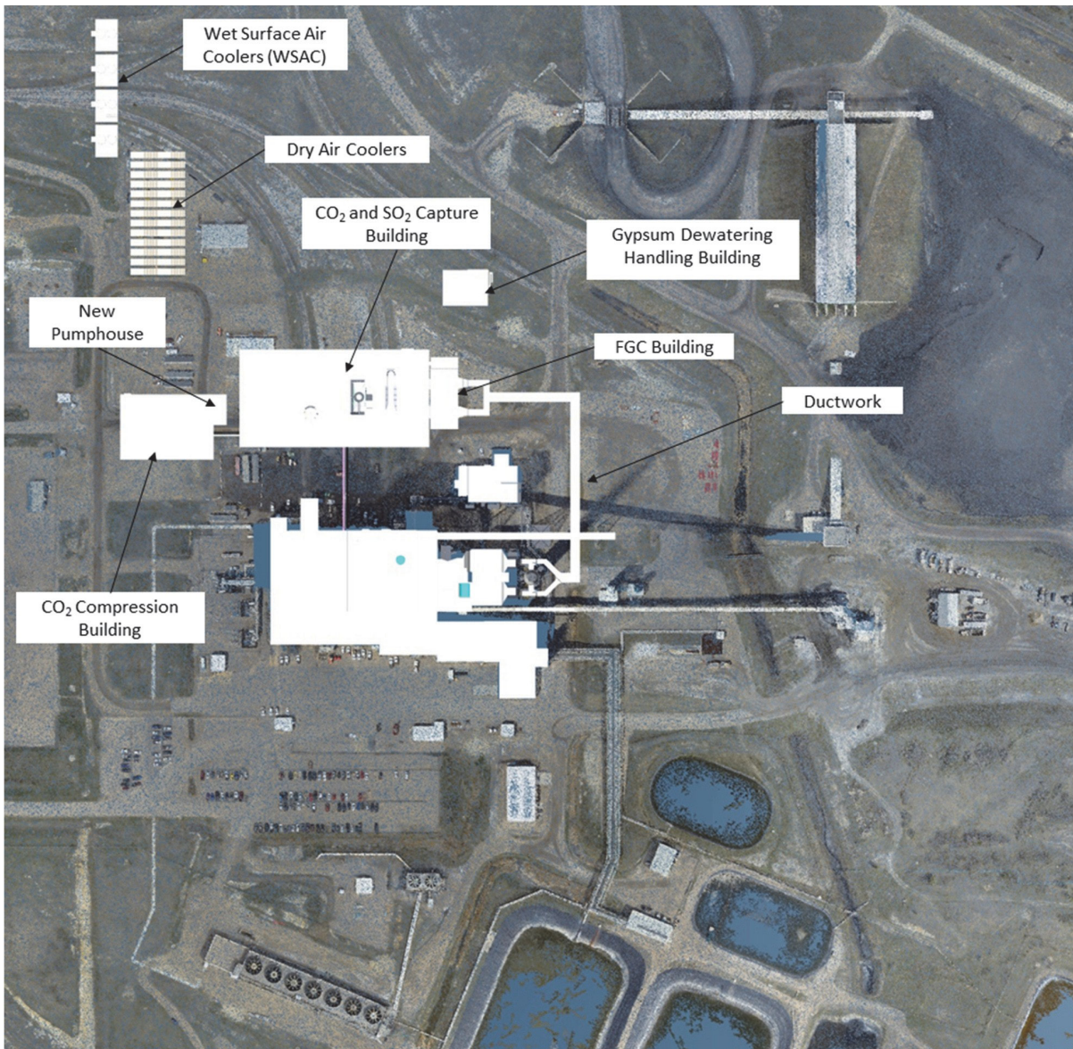
Figure 5.5 Site layout for Shand Power Station with SO 2 and CO 2 capture and heat rejection systems
