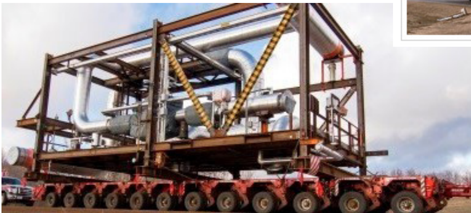
Figure II. Examples of transporting a modularized facility
