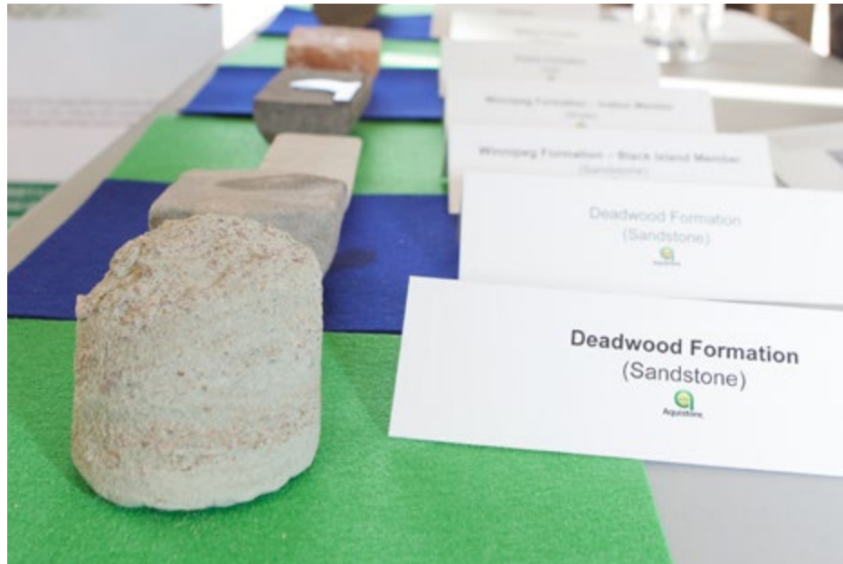
Figure 18. Examining core samples from a drilled well, such as the ones above from southern Saskatchewan, helps to determine how CO 2 will move underground. (Photograph courtesy of the PTRC's Aquistore Project)
