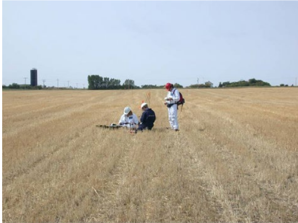
Figure 22. Soil gas samples are taken in a field above the Weyburn oil reservoir. (Photograph courtesy of the PTRC)
