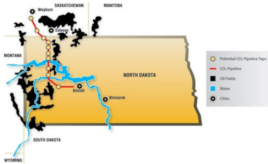
Figure 5. The CO 2 pipeline from Beulah, North Dakota, to the Weyburn oilfield is 320 km long and transports approximately 8000 tonnes of CO 2 per day. (Image courtesy of Dakota Gasification Company)
