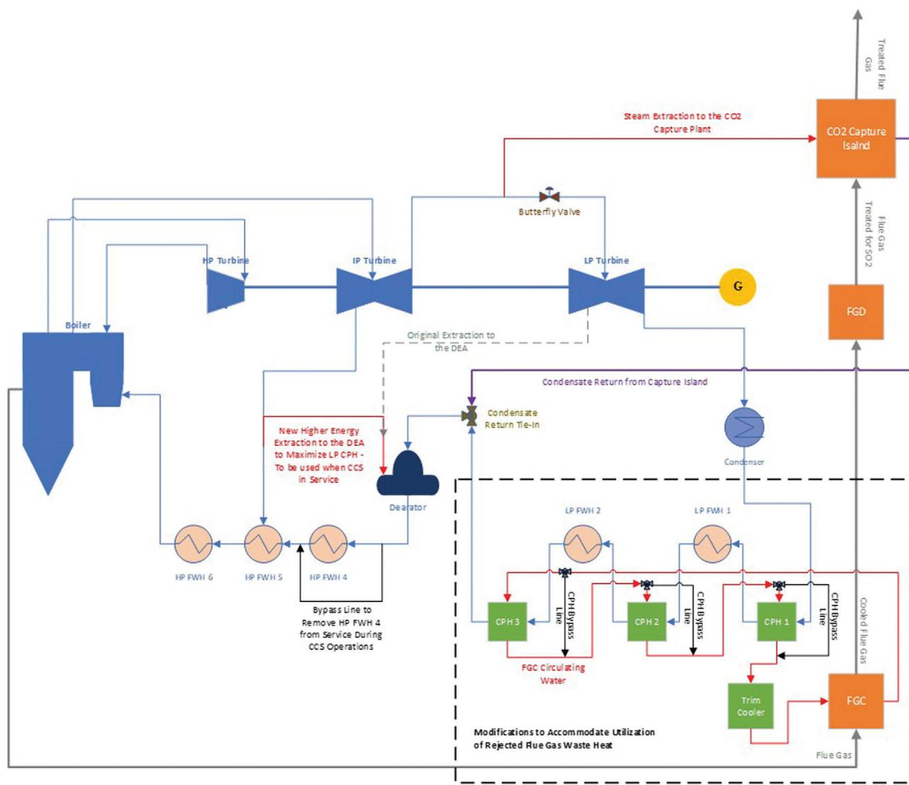
Figure 3. Modifications to the steam cycle to facilitate CCS integration.
