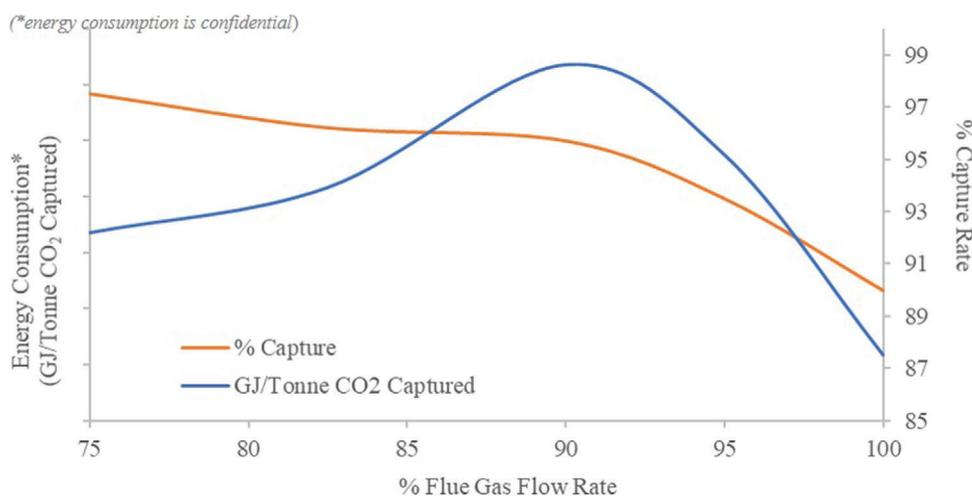
Figure 4. Relationship between energy requirements and capture rate at reduced power plant loads.
