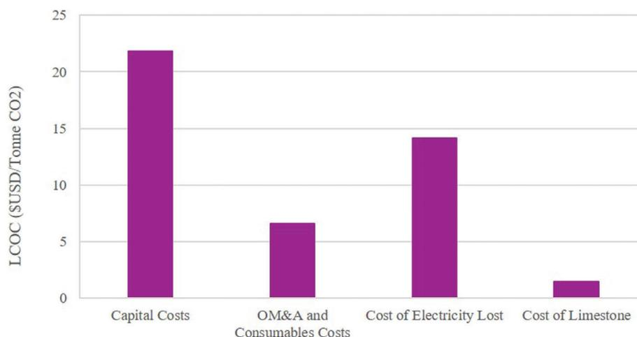
Figure 9. Break down of LCOC for Shand CCS.
