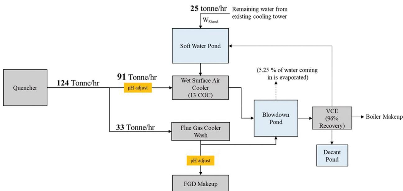
Figure 5. Block diagram of water usage and integration flows for the hybrid cooling system.
