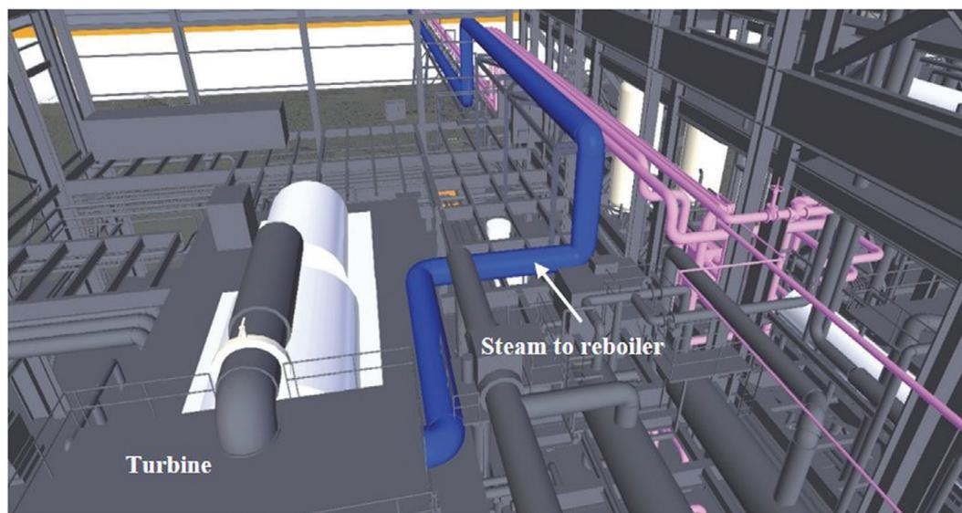
Figure 2. Proposed design and location of the process steam extraction line to the reboiler.
