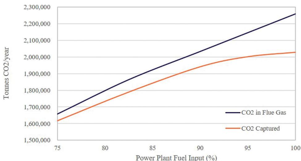
Figure 7. Relationships between CO<sub>2</sub> produced and CO<sub>2</sub> captured with load.
