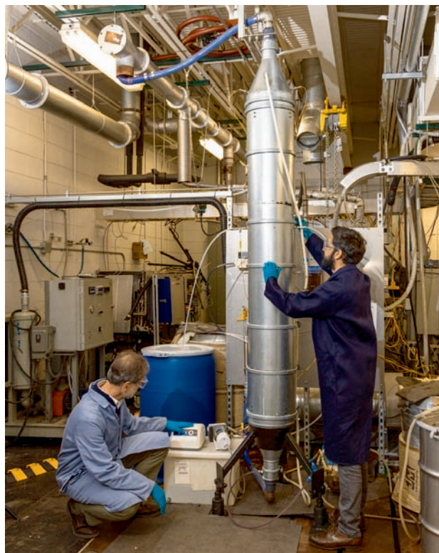
In 2019, ORNL researchers Costas Tsouris and Eduardo Miramontes operated the intensified device inside of the absorption column, which contains commercial stainless-steel packing elements. Credit: Carlos Jones/ORNL, U.S. Dept. of Energy
