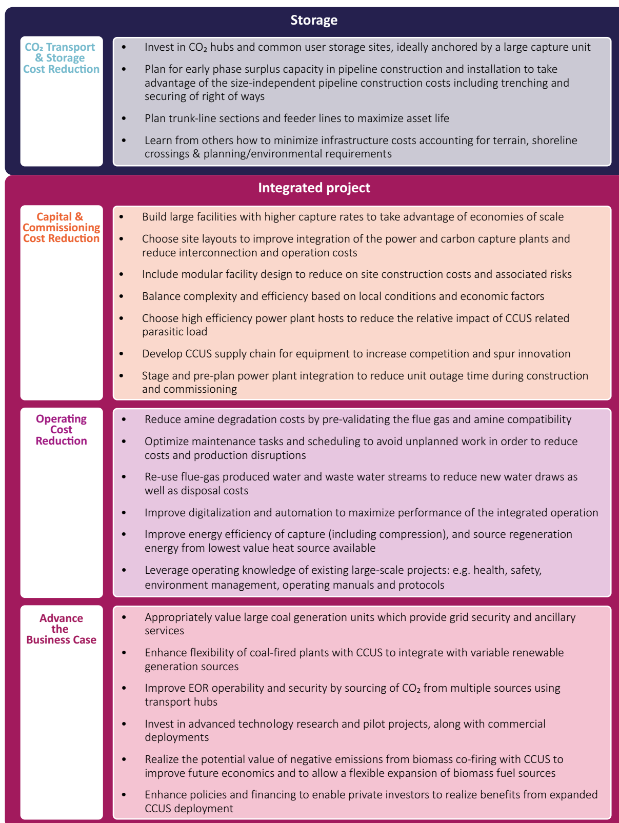
Figure 10: Summary of Cost Reduction Potential for CCUS at Coal-Fired Power Stations
