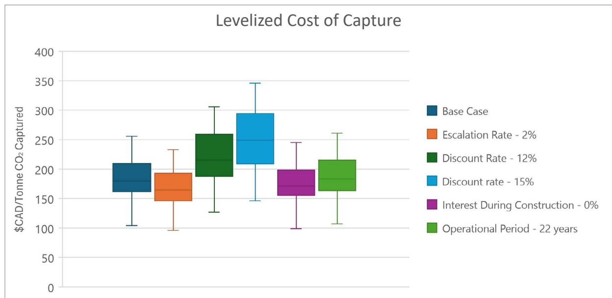
Figure 8: Sensitivity Analysis of Levelized Cost of Capture
